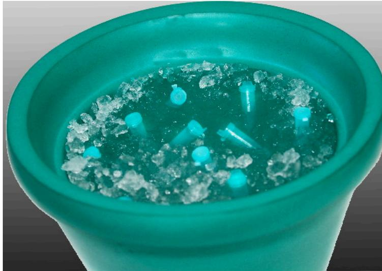
Current method of cooling samples in ice. Directly inserting tubes into ice can result in temperature variability, lost or illegible labels, mis-identification, errors in aliquoting and increased risk of contamination.
